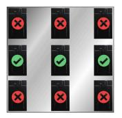
Polarization of Confidex Heatwave Tough is as shown below. This should be considered when using linear reader antennas.
