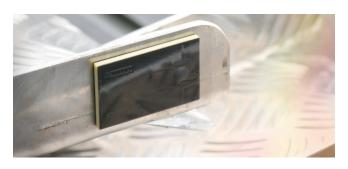
RFID tag with high temperature resistance and good performance for metallic surfaces
